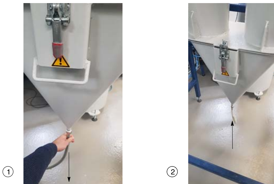
Figure 4 Surge Hopper - blanking the outlet
