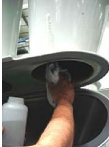
Figure 9 Bottom of cyclone - inspect and clean
