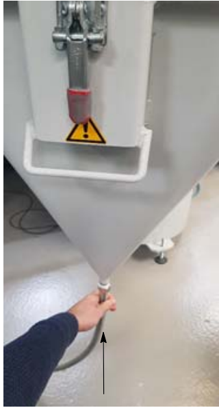
Figure 11 Surge Hopper - reconnect powder transfer hose
