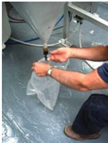
Figure 8 Draining used pellets from surge hopper
