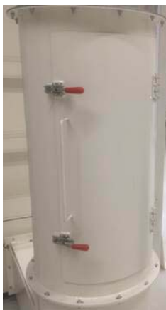
Figure 5 Cyclone Duct Inspection Door - closed & open
